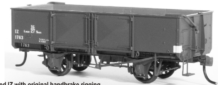
Welded IZ with original handbrake rigging.
