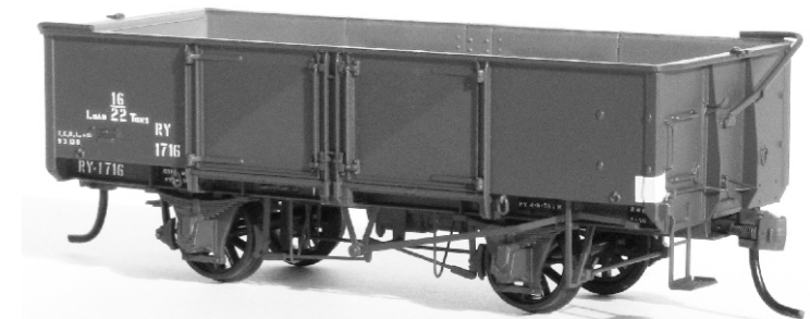
Welded RY wagon with modernised hand brake rigging.
